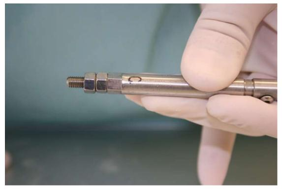
Make sure that nuts D1 and D2 are uncoupled, then turn nut D1 until it is brought in contact with the end of cylinder D: keep tightening it until no more motion is present, thus preventing the nut from being further screwed in (Fig. 5).
